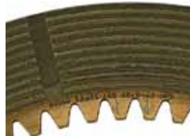
Conoco PowerDrive Profile of grooves still strong despite severe test
