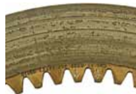
Competitor #1 Heavy wear to plates, grooves worn, deep scratch
