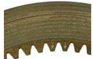
Competitor #2 Extreme wear, almost no profile remains on the friction plate
